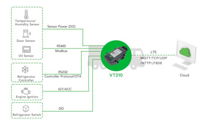
The solution includes cooler equipment, the VT310, a generator set, and the cloud platform. The gateway is connected through RS485 to the sensors of temperature, humidity, oil and doors,
