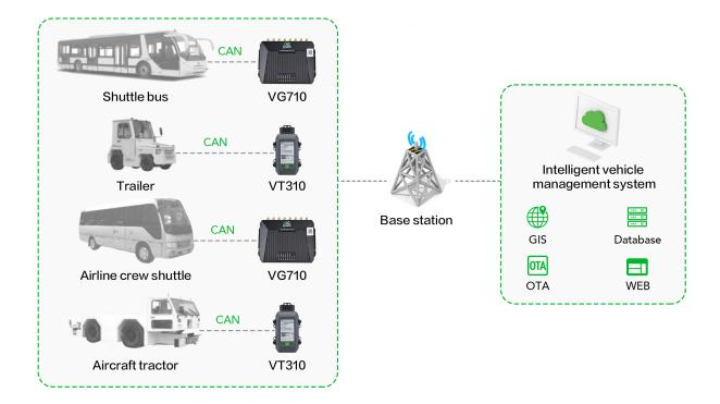
InHand Networks' VG710 smart vehicle gateway connects to the vehicle's ECU and reads related data into the gateway. Real-time vehicle location can be grasped through GNSS positioning and vehicle information is reported to the cloud platform for unified management.
